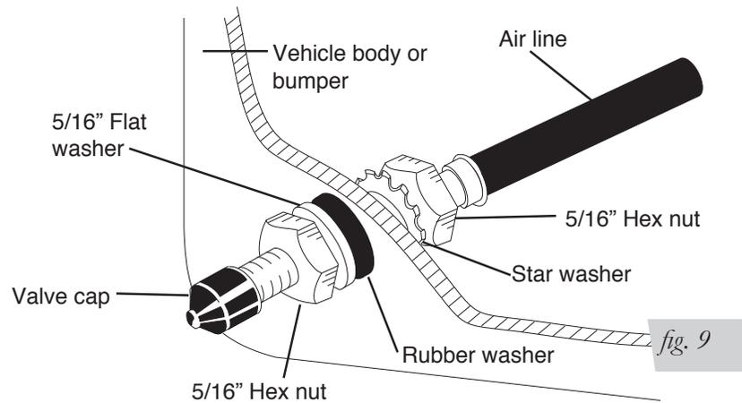
5. Push the inflation valve through the hole and use the rubber washer, flat washer, and another 5/16" nut to secure it in place. Tighten the nuts to secure the assembly.
