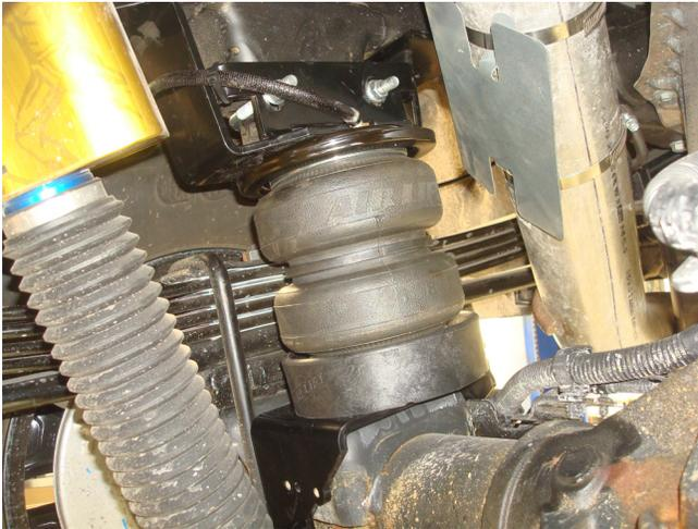
Inside, front of axle view of passenger's (right) side installation.
