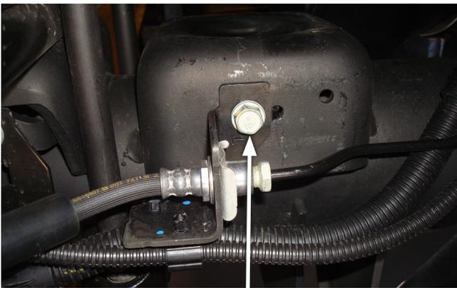
**Remove bolt holding bracket**
