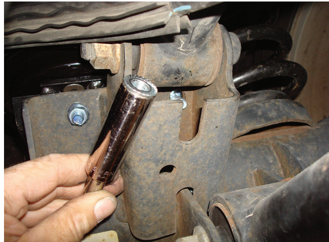
Use the slot in the lower control arm mount for the extension to fit through while threading the nut on the bolt.
