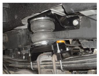
Rear axle view of driver's (left) side installation.
