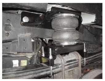
Forward of axle view of driver's (left) side installation.
