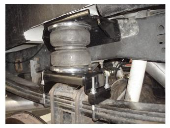
Forward of axle view of passenger's (right) side installation.
