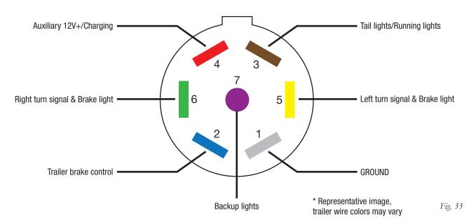
4. Connect the 7-way connector from the trailer (Fig. 33) to the towing vehicle to confirm appropriate connections are being made during the installation.
