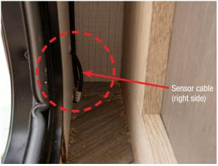
Example of interior routing method used for maximizing *Fig. 29* accessibility to the Sensor cable (right side shown).
