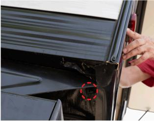
Example of a drilled outlet hole.
