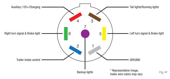
4. Connect the 7-way connector from the trailer (Fig. 41) to the towing vehicle to confirm appropriate connections are being made during the installation.
