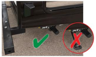
Stow trailer leveling legs before measuring *Fig. 11* for sensor height and leveling
