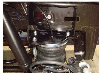
Side view of driver's (left) side installation.
