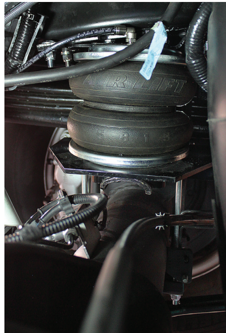
Driver's (left) side inside frame view of kit installed.
