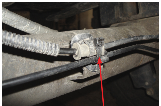
Use a zip tie and attach ABS line to brake line as shown. Fig. 11
