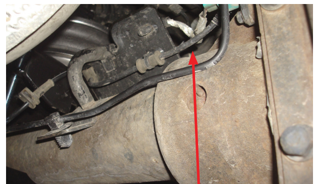
Look for rubbing from modification made to brake components. Adjust where necessary.
