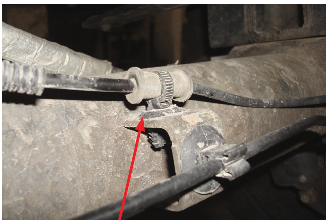
Pull the tree mount holding the ABS line, out of the top mounting of the bracket. Fig. 10
