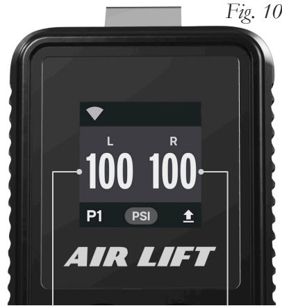
Left Spring Port Pressure Setting
