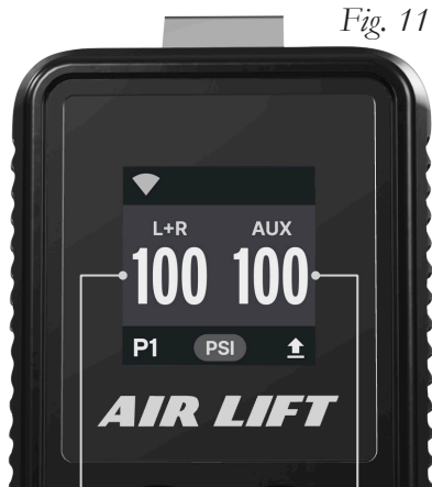
Single Path Pressure Setting
