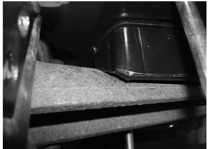
Make sure the cup is seated onto the jounce bumper strike plate forward and behind the axle.
