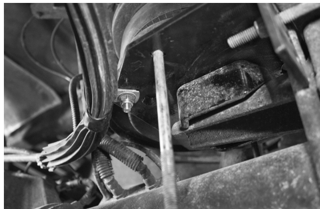
The P-clamp must point down under the lower bracket.
