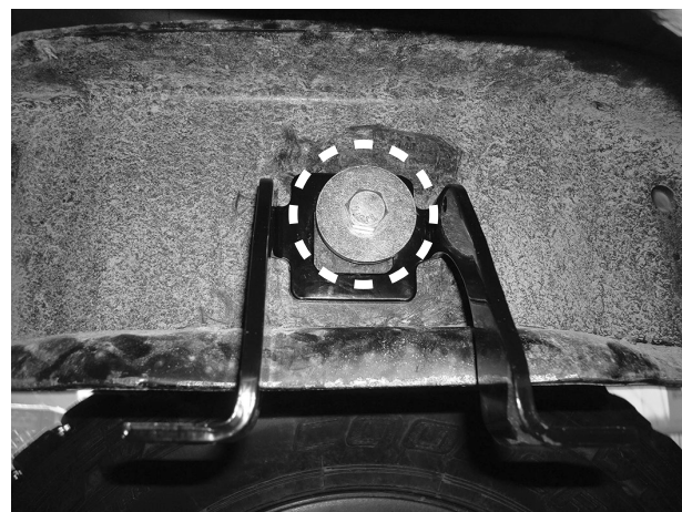
Passenger's (right) side upper brace shown with hardware supplied in place.
