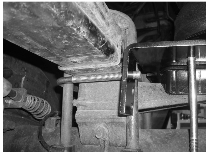
Use closest hole to the leaf spring.
