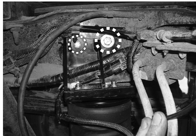
Tighten the M8 hardware and the 1/2" (or 3/4" if from the fifth-wheel hitch hardware) and tighten securely. Repeat for the hardware on the opposite side.
