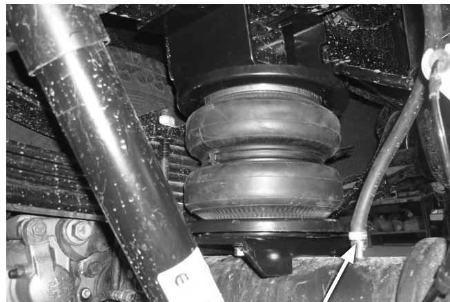
Vent tube fitting and hose
