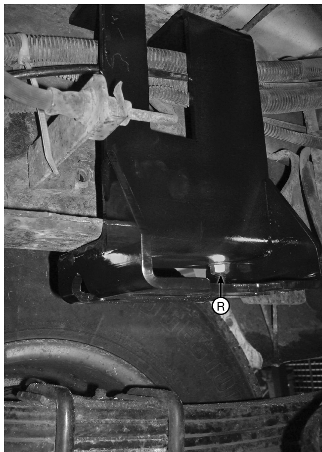
The brake line must not be touching or rubbing the upper bracket.
